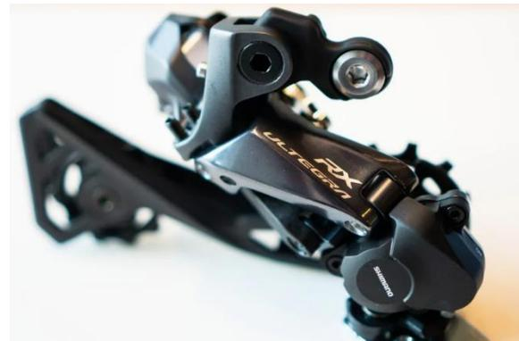
For a minimum of expense and hassle, you can always switch out your derailleur's direct-mount (DM) link with a Wolf Tooth RoadLink DM, assuming your derailleur is a direct-mount (i.e., recent) type; the RoadLink DM fits GRX 810 (RX810), R7000 105, R8000 and RX800 Ultegra and R9100 Dura-Ace rear derailleurs.
