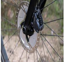
One option to silence squealing brakes is to try a different pad material—just be sure that the rotor does not specify a specific pad material type. *Photo: Dan Cavallari | VeloNews.com*
